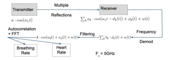
Transmitter: We send high frequency (here, 5GHz) signals from this end.
