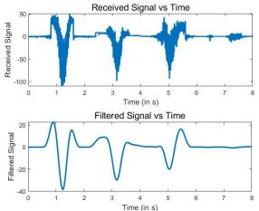
Mathematical Representation:  $y_f(t) = y_f(t-1) + \overline{y}(t)$ ; Thus,  $y_f(t) \approx \sum_k a_k d_k(t) + w_1(t) = a_0 d_b(t) + a_1 d_h(t) + \overline{w}(t)$ ;  $d_b(t)$ -delay caused by breathing;  $d_h(t)$ -delay caused by heart beats.
